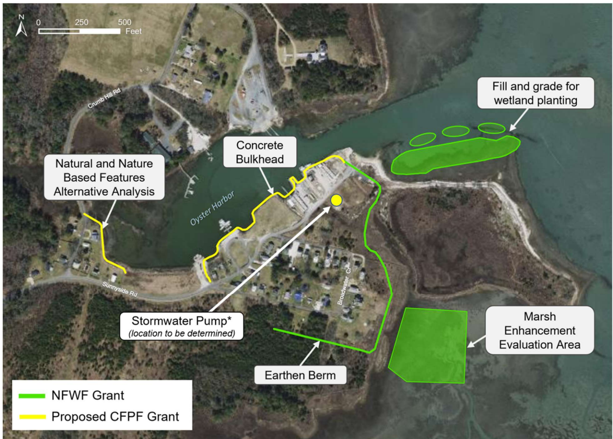
Figure 3: The combination of the NFWF (green) and proposed CFPF (yellow) design elements provide flood protection for Oyster Village. *Location of stormwater pump to be determined during preliminary design.
